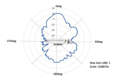
5 GHz Azimuth
