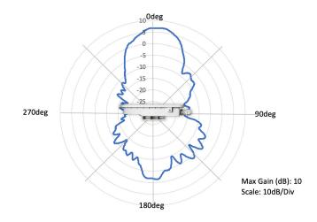
2.4 GHz Azimuth
