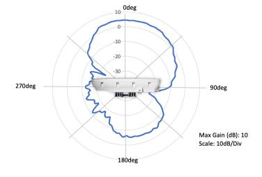
2.4 GHz Azimuth
