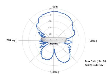
5 GHz Azimuth
